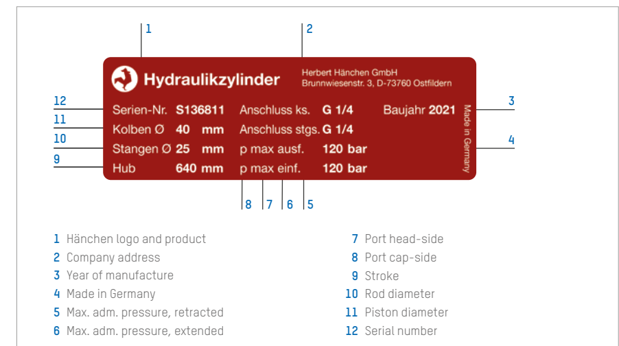
Figure 1: e.g. Type plate of hydraulic cylinder
